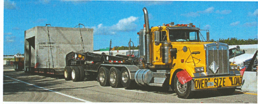
Delivering a 16'x16' precast structure for the I-595 Segment C contract
