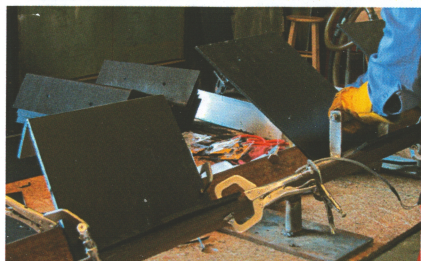
The J-D Shop custom fabricated (above) brackets for skimmers for Hubbard Construction's I-95 ABC and (left) brackets for suspending pipe along a Central Blvd bridge for Murphy Construction.
